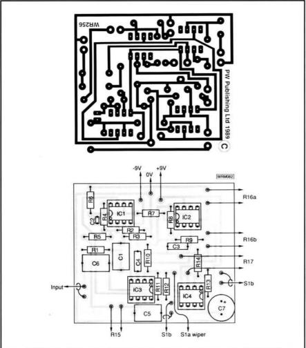
Fig. 1: Single-sided track-pattern and component placement diagram
