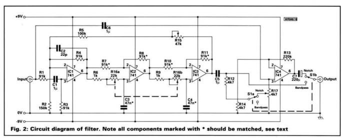
Finally, the high Q at 1kHz, with no apparent ringing, makes the filter ideal for cleaning up c.w. reception and this worked to good effect on the author's transceiver.
