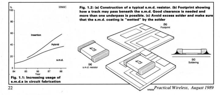
protected by layers of lacquer and a resinous coating. They are largely impervious to moisture and objectionable gases. Surface mount devices on the other hand have little or no protection. Prepared circuits can therefore be sprayed with a protective lacquer - not essential but good practice once a circuit is completed and de-bugged. A solder-through lacquer is the only choice here.
