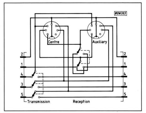
Fig.2.2: Wiring for the Dual Rig Selection Box
